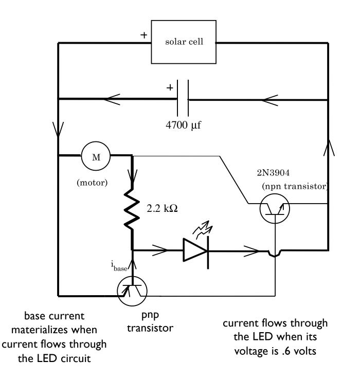
The cap charges. At some point, the voltage across the LED voltage hits .6 volts and current flows through the LED circuit. Current will also flow from the base of the pnp transistor leaving that base electrically negative (relative to its collector). This will turn the pnp transistor "on." This, in turn, turns' on the npn transistor allowing current to flow through the motor unimpeded.
